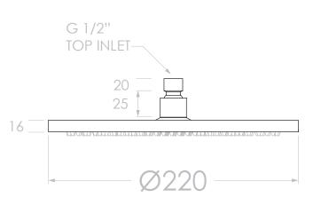
WORKING PRESSURE: 350 – 500KPA (INCLUDING COLD AND HOT WATER PRESSURE)
