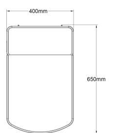
Notice: Rought-in distance should be 150mm if the toilet is against rear wall. Water Pressure: 0.15MPa-0.75MPa(dynamic pressure 1.5-static pressure 7.5kg) minimum flowrate is 5L/8s.
