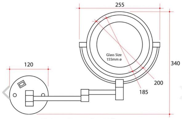
Maximum Distance From Wall 320mm Length From Wall When Folded - 50mm
