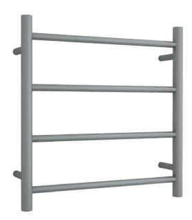
This rail has Multiflex wiring which means that there is a connection point on both the left and right hand side of the rail and the lead can be connected to either side. Being a dry element rail, this can be mounted either way up meaning the wiring can be from any of the four mounting points.
