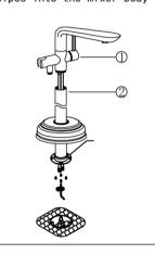
8. Fit floor cover plate onto the extension tube
