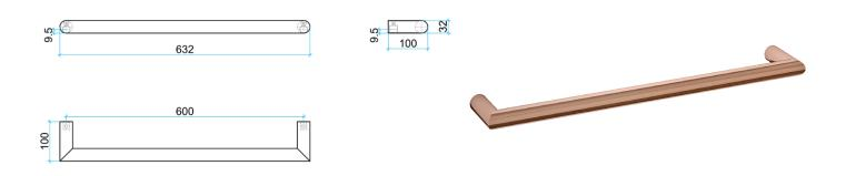
This rail has Multiflex wiring which means that there is a connection point on both the left and right hand side of the rail and the lead can be connected to either side. Being a dry element rail, this can be mounted either way up meaning the wiring can be from any of the four mounting points.
