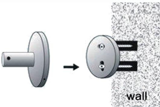
4. Put the base of bathroom accessory cover on the fixing blocks.
