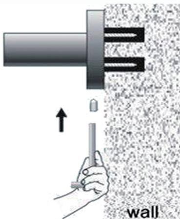
5. Screw grub screws into the base, make it against to the fixing block tight and firm.
