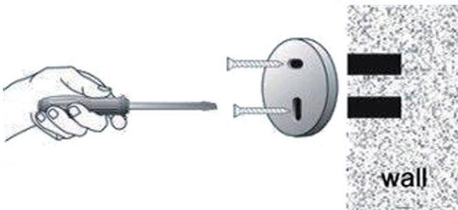
3. Put fixing block cover on the holes and fix firmly by expansion screws.
